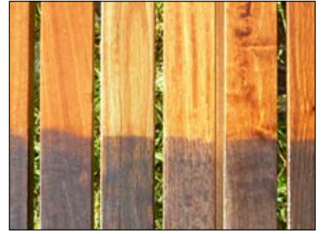
Same piece of timber after a further application of CUTЕКProclean®
